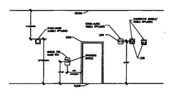
TYPICAL MOUNTING HEIGHT DETAIL FOR WALL-MOUNTED COMPONENTS
